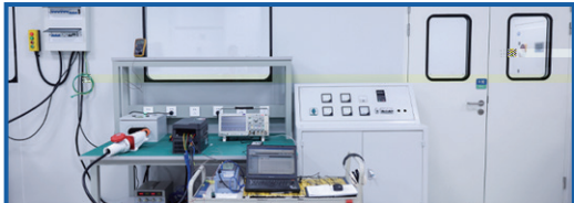
Switching Power Supply Testing Platform
